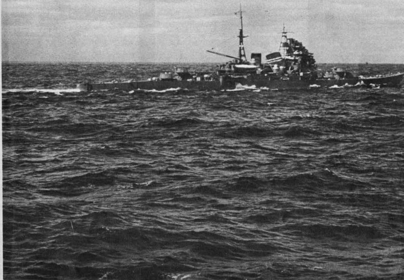
Powerful Atago Class cruiser swings its five twin turrets to port for a broadside. Japanese sacrifice everything to favorable battery arrangement; hence concentrated, and crowded superstructure. Since
